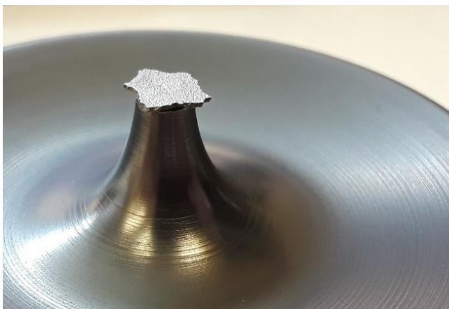
Fig. 3 – Sputter source holder A graphite pedestal supports an 8.9 mg flake of enriched Ru-102.
